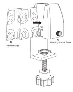
STEP 3: Fit Mounting Brackets (Part B) to the edge of the table top and turn Tension Knob clockwise to tighten.
