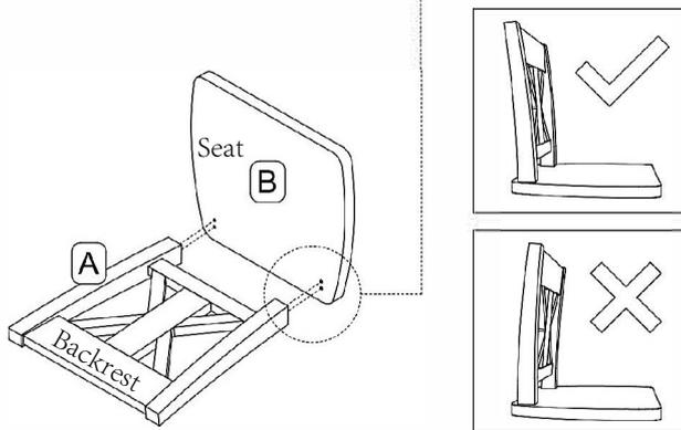
Attach the Backrest (Part A) to the Seat (Part B) using (4) M6x45mm Hex Screws (Part 3), (4) Lock Washers (Part 4) and (4) small Flat Washers (Part 6). Tighten loosely with Allen Wrench (Part 7).
