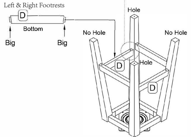
Attach Left & Right Footrests (Part D) to the large holes on the Chair Legs (F & G) using (4) M4x38mm Phillips Screws (Part 1). Tighten loosely with Phillips Screwdriver (Not Included).
