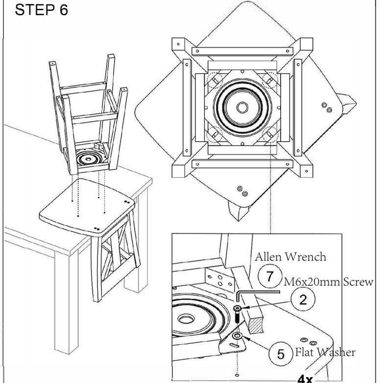
Invert the assembled backrest and seat on a stable raised surface such as a table. Attach the Swivel Plate located on the Apron with Swivel Plate (Part E) to the Seat using (4) M6x20mm Hex Screws (Part 2) and (4) Flat Washers (Part 5) Tighten all screws using the Allen Wrench (Part 7). Return Chair to the upright position.
