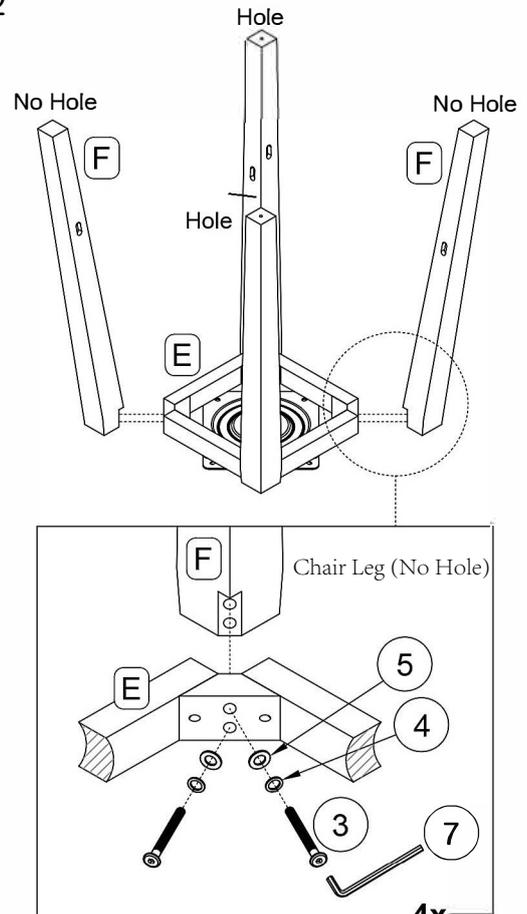
Attach (2) Chair Legs with Hole (Part G) on opposite sides of the Apron with Swivel Plate (Part E), using (4) M6x45mm Hex Screws (Part 3), (4) Lock Washers (Part 4) and (4) Flat Washers (Part 5). Loosely tighten with Allen Wrench (Part 7).
