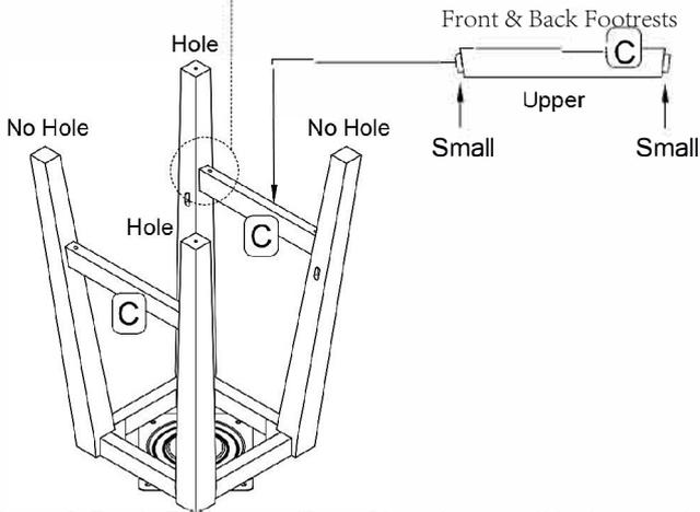
Attach Front & Back Footrests (Part C) to the small holes on the Chair Legs (F & G) using (4) M4x38mm Phillips Screws (Part 1). Tighten loosely with Phillips Screwdriver (Not Included).
