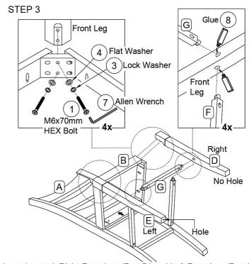
Loosely attach Right Front Leg (Part D) and Left Front Leg (Part E) to Box Frame (Part B) using (4) M6x70mm Hex Bolts (Part 1), (4) Lock Washers (Part 3), and (4) Flat Washers (Part 4). Apply Glue (Part 8) to the lower holes in the Front Legs and insert Footrest (Part G) and Left and Right Side Braces.
