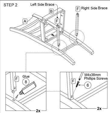
Apply some Glue (Part 8) to the bottom holes of the Chair Back (Part A) and insert the Left and Right Side Braces (Part F). Insert (2) M4x38mm Phillips Screws (Part 6) and tighten using a Phillips Screwdriver (not included). **Do not fully tighten screws in this step.**
