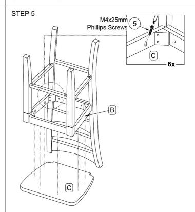
Attach Wooden Seat (Part C) and Box Frame (Part B) using (6) M4x25mm Phillips Screws (Part 5). Securely tighten using Phillips Screwdriver (not included).
