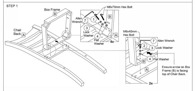
Lay the Chair Back (Part A) on its back and attach Box Frame (Part B) using (4) M6x70mm Hex Bolts (Part 1), (4) Lock Washers (Part 3), and (4) Flat Washers (Part 4). Loosely tighten using Allen Wrench (Part 7). Insert (2) M6x40mm Hex Bolts (Part 2), (2) Lock Washers (Part 3) and (2) Flat Washers (Part 4) into the predrilled holes of the middle of Chair Back (Part A). Tighten using Allen Wrench (Part 7). **Do not fully tighten the bolts in this step.**
