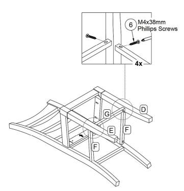
Insert (4) M4x38mm Phillips Screws (Part 6) into the holes Side Braces (Part F) & Front Footrest (Part G). Securely tighten using Phillips Screwdriver (not included).
