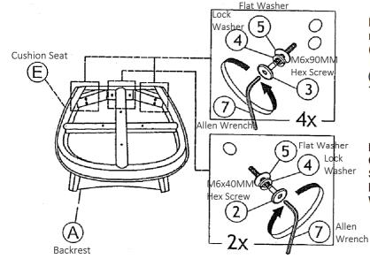
Invert Cushioned Seat (Part E) and place on a stable raised surface such as a table. Attach the Backrest (Part A) to the Cushioned Seat (Part E) using (4) M6x90mm Hex Screws (Part 3), (4) Lock Washers (Part 4), and (4) 6.5x16.5mm Flat Washers (Part 5). Tighten using Allen Wrench (Part 7).
