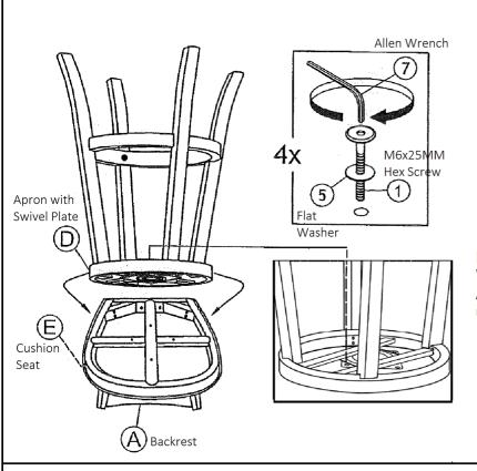
Keep the Backrest (Part A) and Cushioned Seat (Part E) inverted on a stable raised surface. Attach the Swivel Plate located on the Apron with Swivel Plate (Part D) to the Cushioned Seat (Part E) using (4) M6x25mm Hex Screws (Part 1) and (4) 6.5x16.5mm Flat Washers (Part 5) Tighten all screws using Allen Wrench (Part 7). Return Chair to the upright position.
