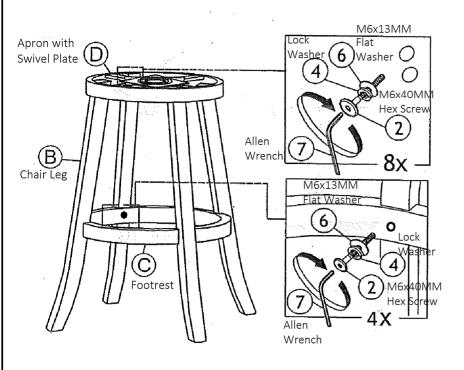
Attach the Chair Legs (Part B) to the Apron with Swivel Plate (Part D), then attach the Footrest (Part C) to inside of the Chair Legs (Part B) using (12) M6x40mm Hex Screws (Part 2), (12) Lock Washers (Part 4) and (12) M6x13mm Flat Washers (Part 6). Loosely tighten using Allen Wrench (Part 7).
