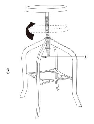
To rotate the screw mandrel into the metal frame; then to insert the spring pin on the bottom of the screw mandrel.
