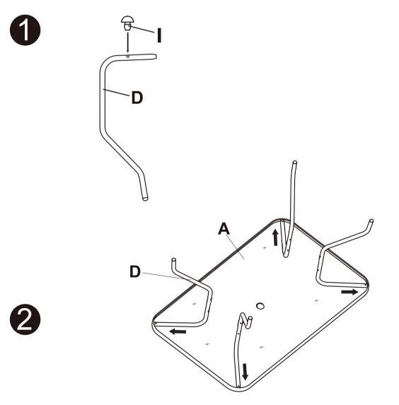
Note: The plastic leg sleeves are adjustable to the left or right, please slide them to the corners before attaching the legs
