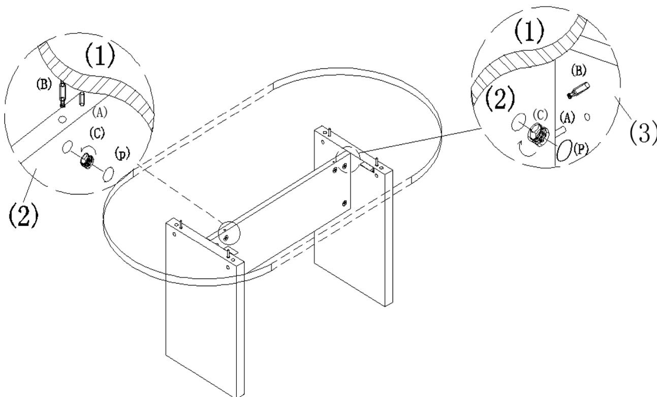
Attention: Please apply Part (P) Cam Covers over each exposed Part (C) Cam Lock after finishing the installation.
