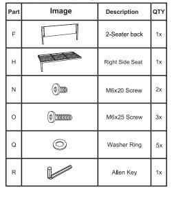
STEP 3 A: From inside of the frame, attach 2-Seater Back (Part F) to Right Side Satt (Part H) using (3) Washer Rings (Part Q) and (3) M6x25 Screws (Part Q). Do not tighten completely
