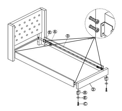
Loosen the screws (Part A) pre-assembled in the side rail (Part 3). Attach the side rail then tighten the screws.
