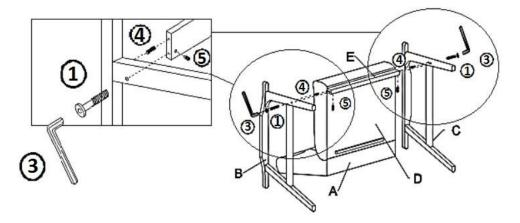
Insert Wood Dowels (Part 4) into the Seat Rail (Part E) as pictured to the left.
