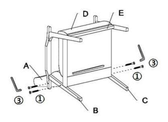
Attach Backrest (Part A) to Right Arm Panel (Part C) and Left Arm Panel (Part B) using JCBC Bolts (Part 1) with Allen Wrench (Part 3).
