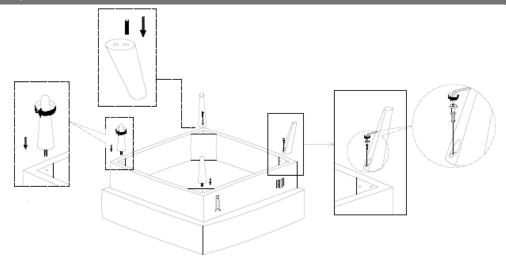
Insert the Front Legs into the underside of the Chair Seat and turn clockwise to tighten. Insert Dowel Rods already assembled in Rear Legs (Part 5) into the bracket on the underside of the Chair Seat. Using (2) M8 x 60MM Bolts (Part A) and (2) Lock Washers (Part B) complete the installation of the Rear Legs. Tighten using an Allen Wrench (Part C).
