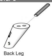
Insert (1) Wood Dowel (Part D) into the upper hole in Back Legs (Part 5)
