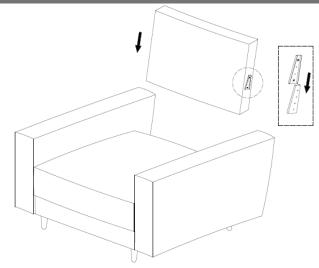
Slide the brackets on the Back Panel into the receiver brackets on the inside of Right Side Panel and Left Side Panel.
