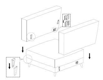
Return chair to the upright position and insert the brackets on the Right Side Panel and Left Side Panel into the receiver Brackets on the side of the chair.
