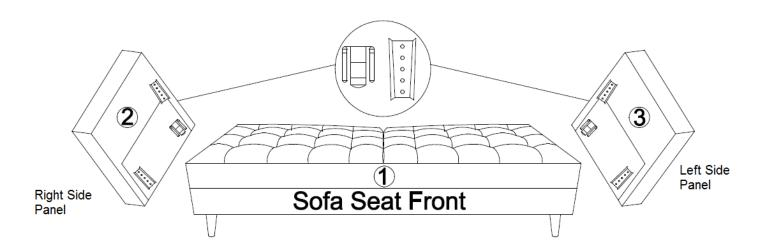
Return sofa to the upright position and insert the brackets on the Right Side Panel (Part 2) and Left Side Panel (Part 3) into the receiver Brackets on the side of the sofa.
