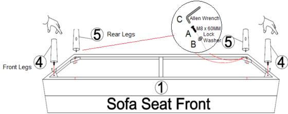
Insert the Front Legs (Part 4) into the underside of the Sofa Seat and turn clockwise to tighten. Insert Dowel Rods already assembled in Rear Legs (Part 5) into the bracket on the underside of the Sofa Seat. Using (2) M8 x 60MM Bolts (Part A) and (2) Lock Washers (Part B) complete the installation of the Rear Legs. Tighten using an Allen Wrench (Part C).
