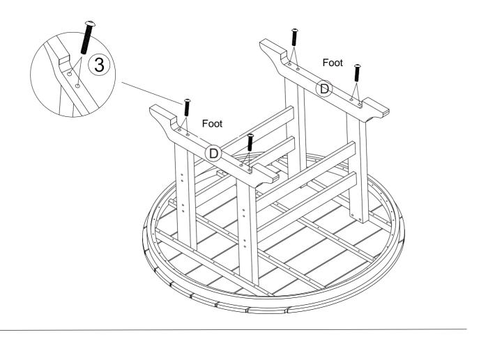
STEP 4: Ensure all screws are securely tightened.
