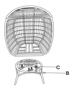
From the underside of the base, attach the rotating turntable plate to the basket using (4)M6\*20Screws (PartC) with washer (Part E) on the inside. Tighten using Allen Wrench
