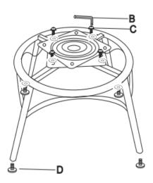
Align the turntable with the screw holes on the base and attach using (4)M6\*20 Screws (PartC). Tighten using Allen Wrench (Part B). Insert the Floor Glides (Part D).
