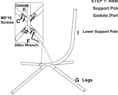
STEP 1: Attach (4) Legs (Part G) to the lower half of the Support Pole (Part I) using (8) M8\*16 Screws (Part C) and (8) Gaskets (Part K) Tighten using Allen Wrench (Part F).
