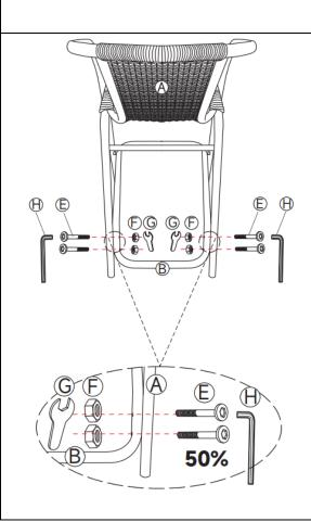
STEP 3 Completely tighten all screws.
