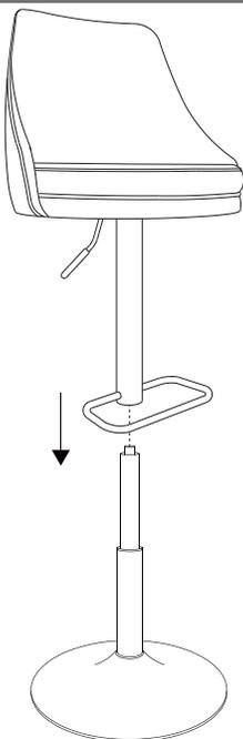
Insert the assembled Seat and Pedestal Base onto the Gas Lift Cylinder.
