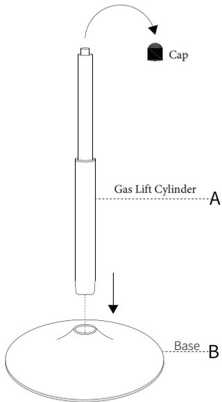
Remove the cap from the Gas Lift Cylinder and discard. Insert Gas Lift Cylinder firmly into the Base (Part B).
