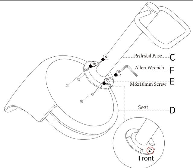
Align the holes in the Pedestal Base (Part C) with the holes in the underside of the Seat (Part D). Attach using (4) M6x16mm Screws (Part E). Ensure the arrow on Pedestal Base plate is facing the front of the seat.
