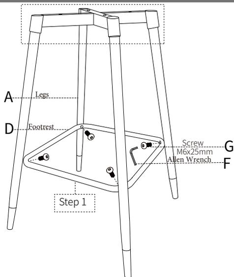
Align the holes on the Footrest (Part D) with the holes on the Legs (Part A). Attach using (4) M6x25mm Screws (Part G). Tighten using Allen Wrench (Part F). After installation of Footrest, completely tighten screws from Step 2 in the Leg Connectors.
