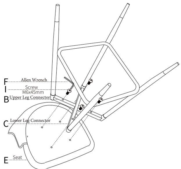
Align the holes on the underside of the Seat (Part E) with the holes in the Upper and Lower Leg Connectors (Parts B & C). Attach using (4) M6x45mm Screws (Part I). Tighten using Allen Wrench (Part F).
