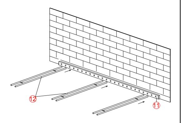
**Step 3b:** Insert part 13 pieces into the holes in part 11.
