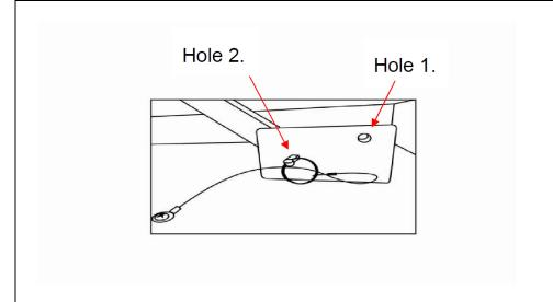
Step 2: Insert the pins into Hole 2.
