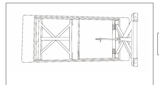
**Step1:** Open the box and remove the security pins from Hole 1, then open the legs.
