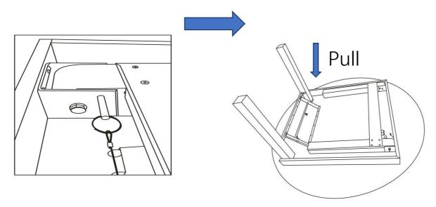
STEP 3: Insert the same pins back into position to lock the four legs during use.
