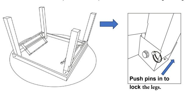
NOTE: Do not use the table unless the security pins are inserted and the table is steady.
